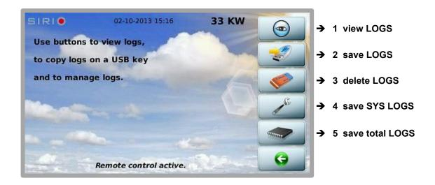
To **view the logs**, press the button with the symbol. Then select the measurements to be displayed (only two measures can be displayed at the same time):
