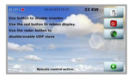
The first button allows you to disable the inverter and re-enable it.
