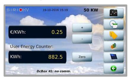
On this screen, you can manually set the €/kWh ratio and reset the partial hour meter for the energy produced.
