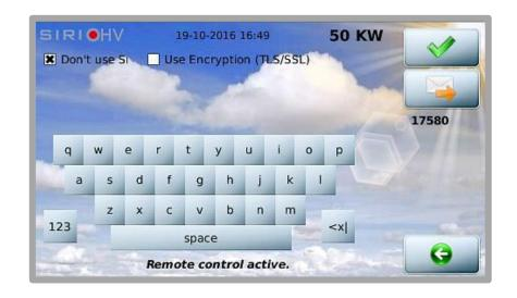
At the end of the configuration procedure, it is possible to send a test e-mail message to verify whether the settings are correct, by pressing the button.
