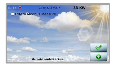
If the function Extern Modbus Measure is selected, a set of default parameters are presented. These parameters are prepared for the external instrument given by Aros Solar. Anyway it's possible to connect other brand instruments on the 485 bus; in this case an accurate reading of the manual is suggested to have the correct settings:
