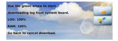
The button allows the user to download the logs of the system board and of the display on USB key. Use the same procedure seen before.
