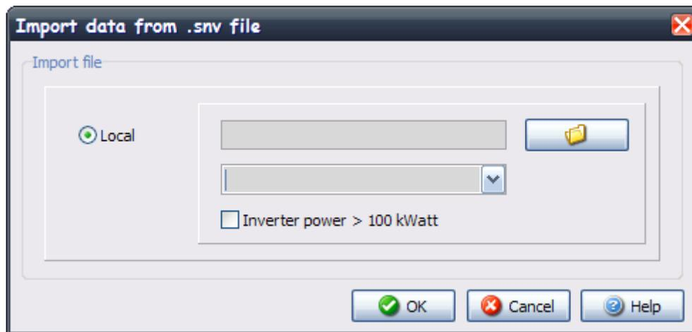
Local: this section allows you to convert .snv data files recorded by the Sunvision1 program and make them compatible with data files created by the Sunvision2 program. In this section, you will have to select the file you want to import and the inverter that the file is associated with.
