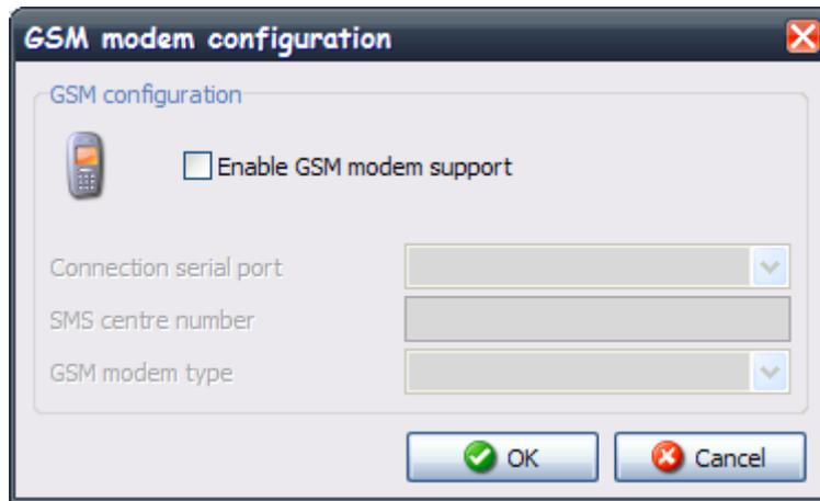
Enable GSM modem support: enable or disable GSM modem support. When disabled, the **PVMON** cannot send SMS.
