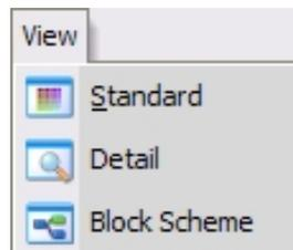
**Standard view:** in the graphic (Standard) visualization will be shown three measures: percentage power network, DC Voltage (three-phase or mono-phase depending on inverter); internal inverter temperature.
