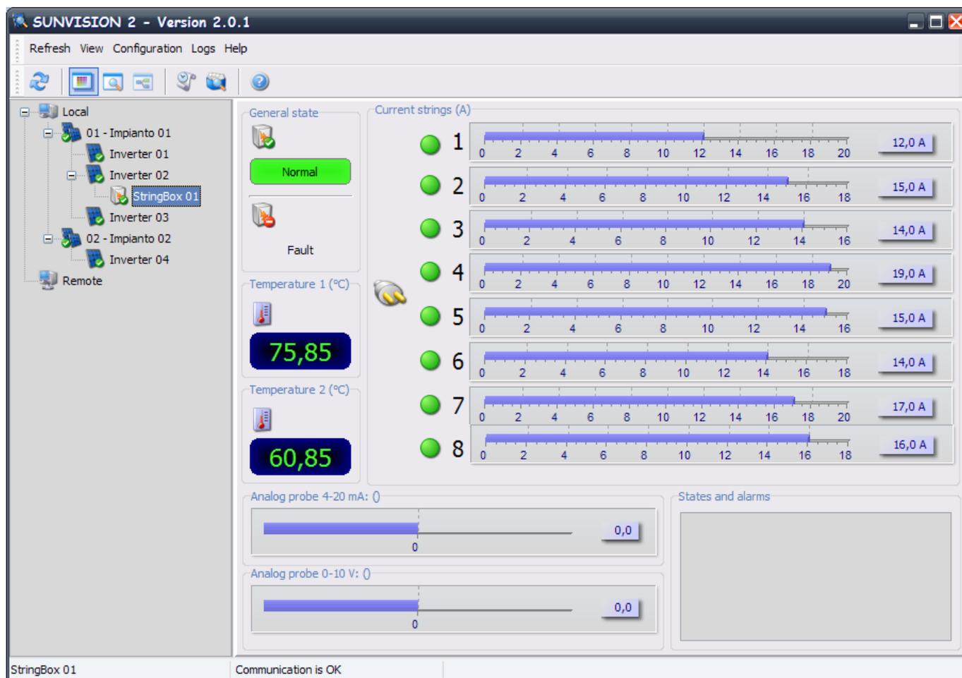
**General State:** it is shown the Stringbox complete status. The colours show the status of the StringBox. The two states can be: normal (green) - works ok, Fault (Red) - StringBox in Fault status.
