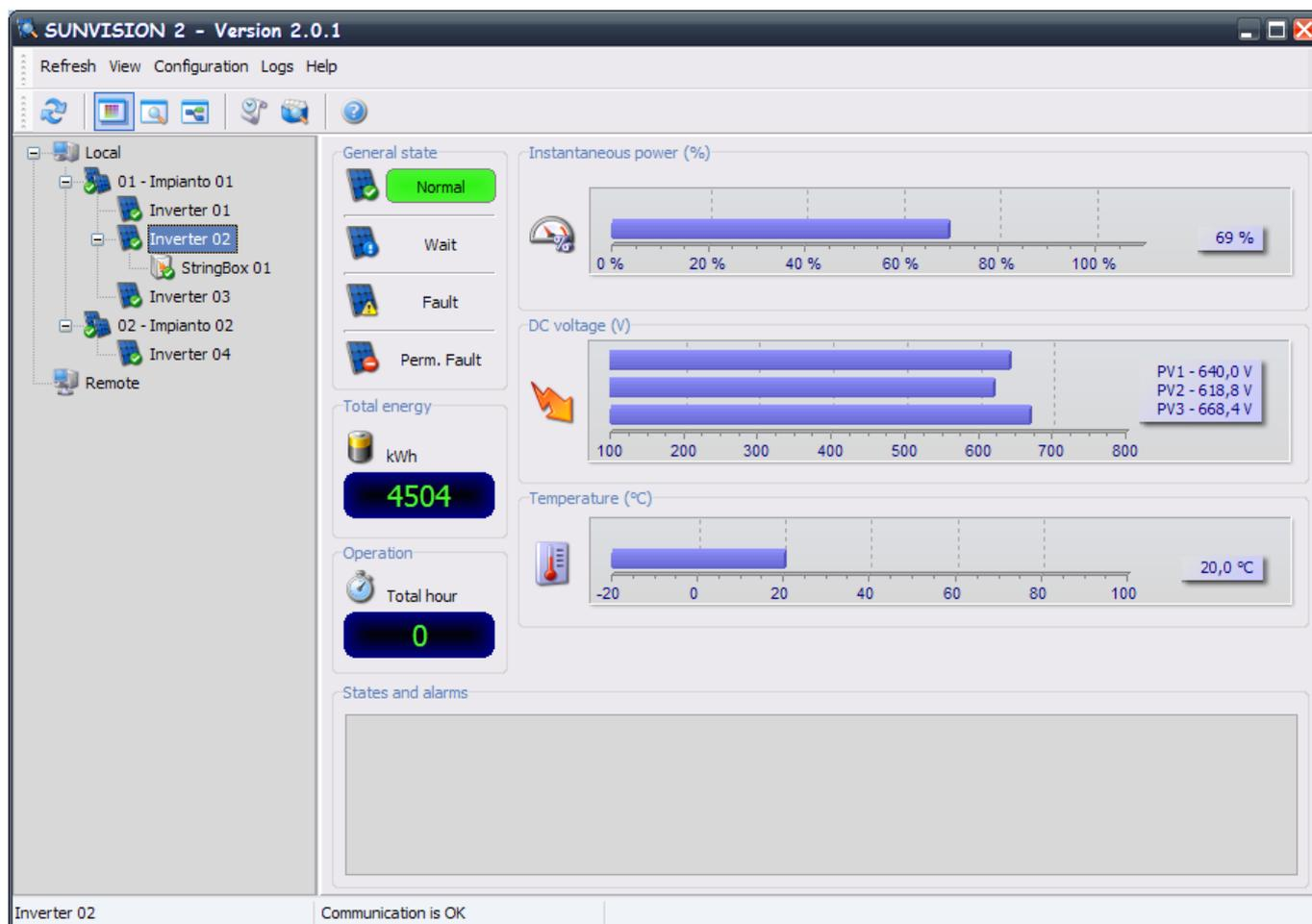
**Detail view:** in the numeric (Detail) visualization will be shown all of the detailed information with regards to the measured values from Inverter.
