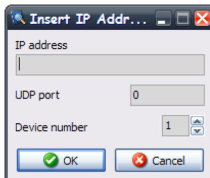
You may choose Inverter directly by IP address of computer or SNMP adapter, where is connected Inverter. For this you must set IP address, UDP Port and device number (usually 1). The *Pvview* will try to find the specified system by IP address. The host names or DNS names is also supported.
