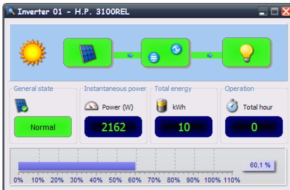
In these windows you can have a full view of the state of the inverter. You can see the block scheme of the inverter, the general state, the instantaneous power, the total energy, the operation hours and a graph representing the instantaneous power in percentage.
