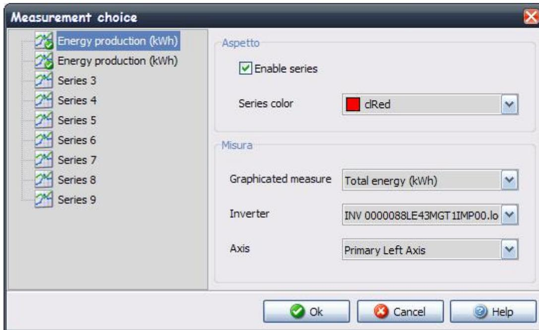
Tree : the tree on the left shows the nine series that can be displayed on the graph. The green check on the icon of the series, indicates that the series is already active and associated to some measure.
