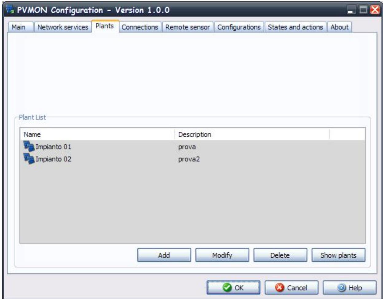
The maximum number of configurable plants is 64. The plants can be added, changed or eliminated with buttons. A special button "Show System" will see the pattern of plant and the associated inverter.
