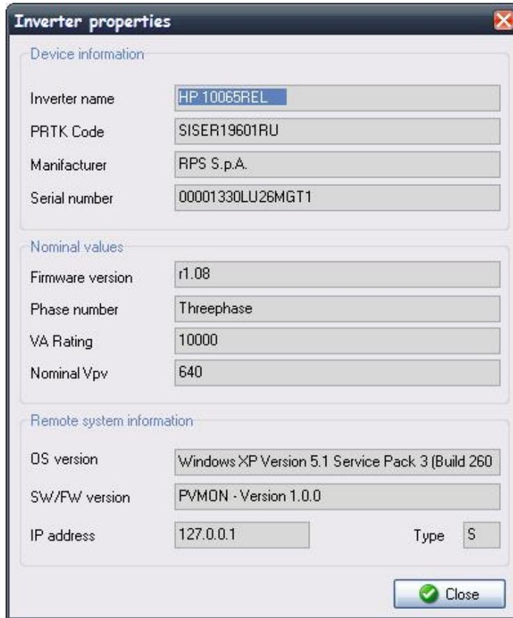
From this window you can see the properties of the monitored Inverter such as name of Inverter, connection type, the type of communication protocol, some information on Pvagent or SNMP adapter that controls it and some nominal data of the device.
