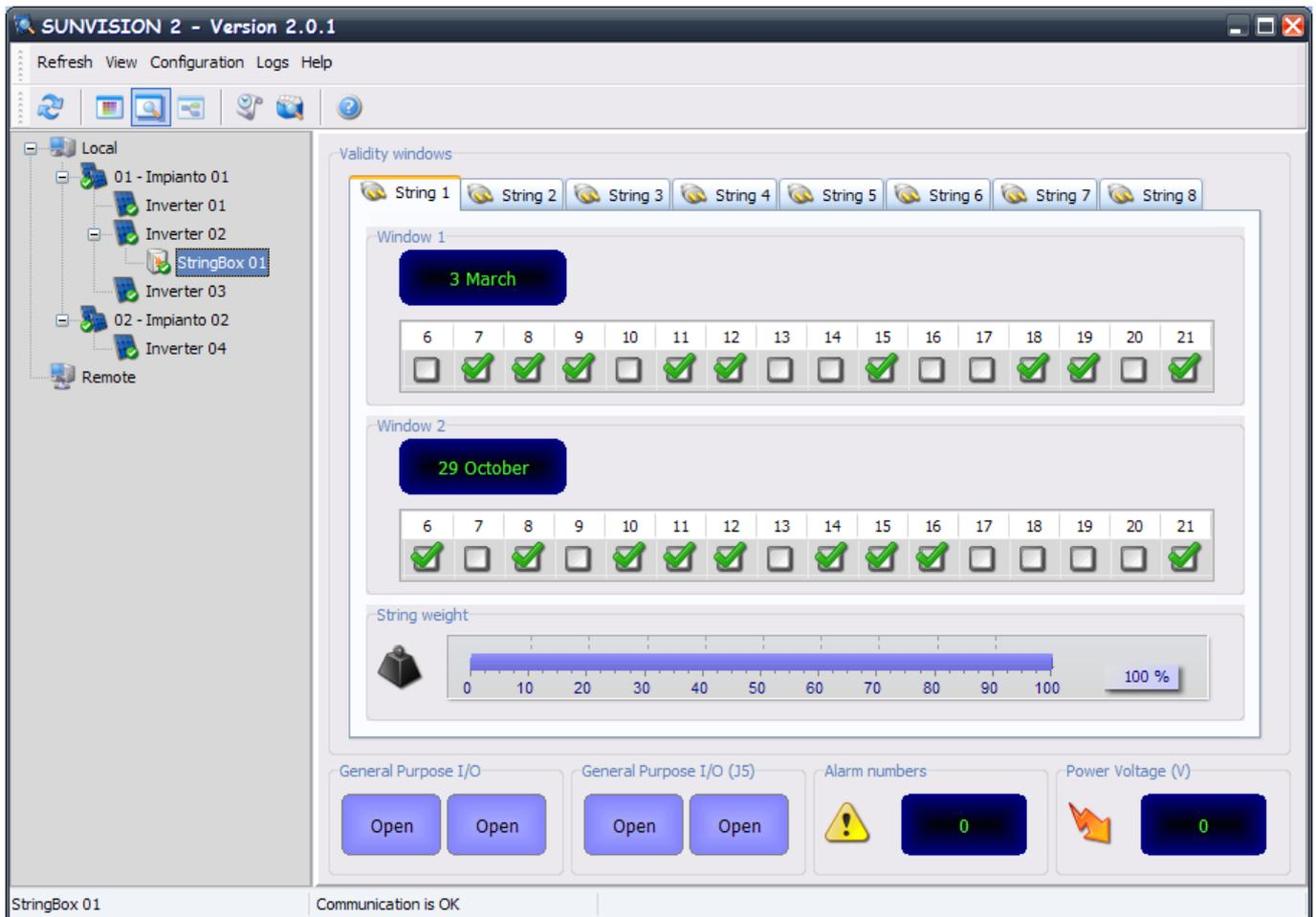
In this view you can see the validity windows set on the various current strings of Stringbox. The validity window is from 7 to 22 hours and can be configured each single hour. The windows are two, and come into play on the date shown in the box.
