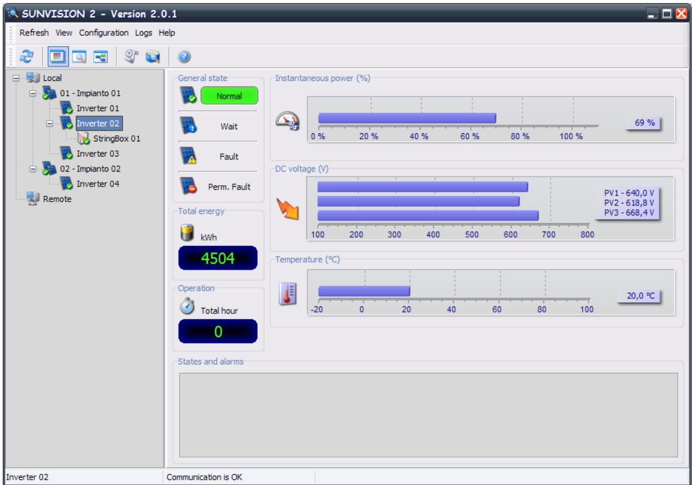
**General State:** it is shown the Inverter complete status. The colours show the status of the Inverter. It can be four state: Normal (green) - Inverter is OK and working; Wait (yellow) - Inverter is in wait state; Fault (red) - Inverter is in Fault state; Perm. Fault (red) - Inverter is in permanent fault state.
