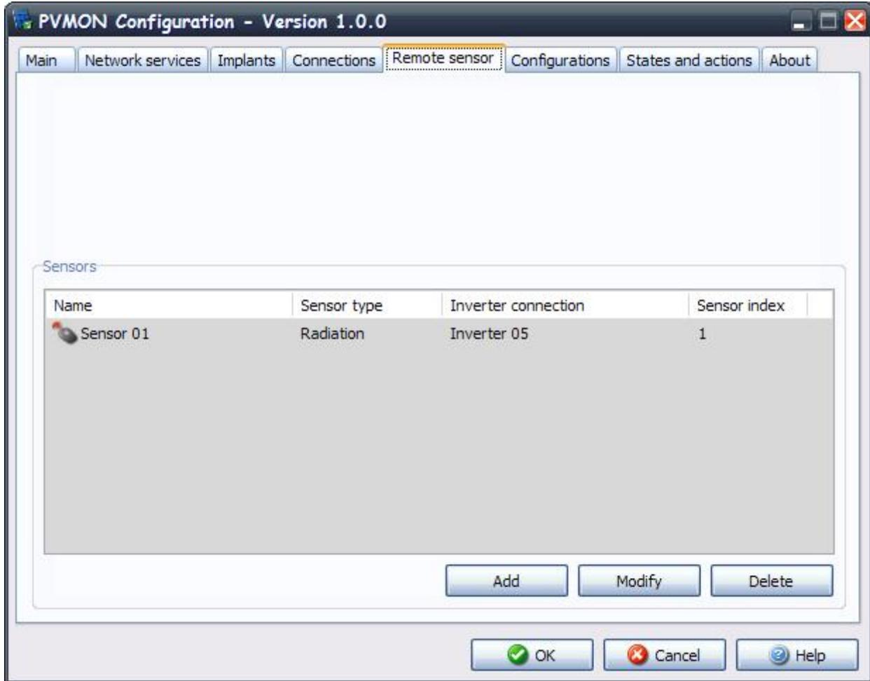
This window shows the list of remote sensors associated with the SNMP adapter connected to the Inverter. Up to 6 different types of remote sensor can be associated with an SNMP adapter using the serial port (see sensor cable wiring specifications). The remote sensors are divided into four categories:
