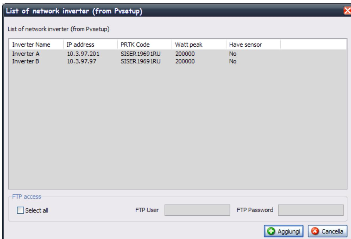
From this list, you can select (by means of single/multiple selection or checking the Select All box) the inverters that will be added to the Netman or Display lists according to which Add button has been pressed.
