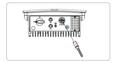
Step 5 Remove an appropriate length of the insulation layer from the PV Strings power cables.
