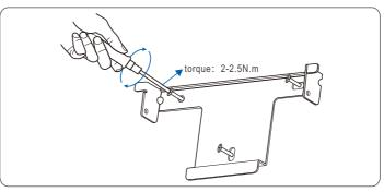
Step 6 Mount the inverter on the rear panel and tighten the screws at both sides.
