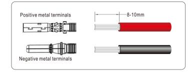
Step 6 Insert the exposed areas of the positive and negative power cables into the metal terminals of the positive and negative connectors respectively and crimp them using a crimping tool.(Connect the red wire to the positive metal terminal, and the black to the negative.)
