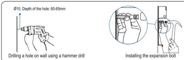
Step2 Tighten the expansion screw.
