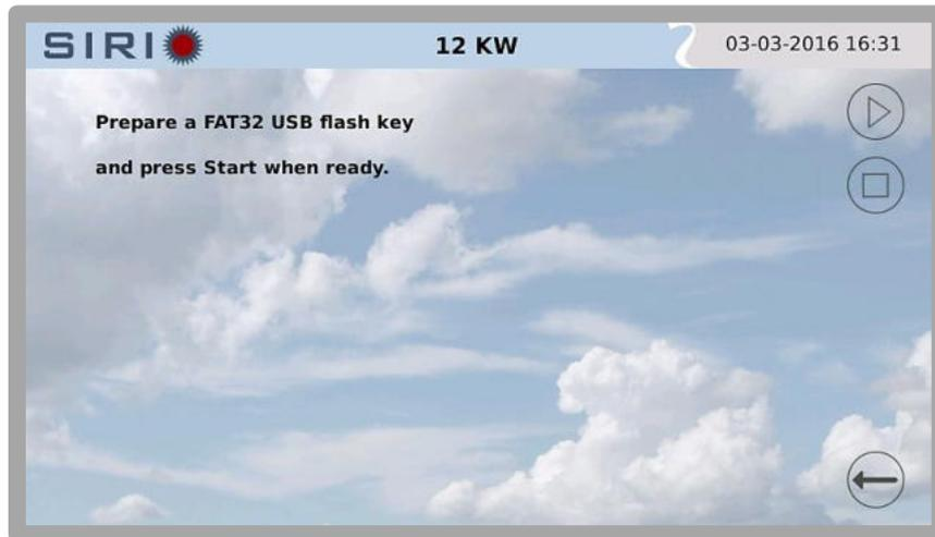
As mentioned previously, the USB flash drive must be formatted in FAT32 (VFAT) and have a single partition. Many USB flash drives containing dedicated security software with special partitioning schemes may not work.
