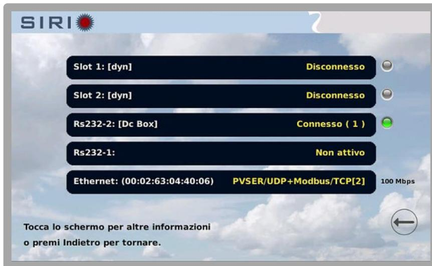
The above example shows a PVSER/UDP and Modbus TCP connection on the Ethernet port and a connection to an external reading on serial port no. 2, which in this case corresponds to the DC-BOX current readings.
