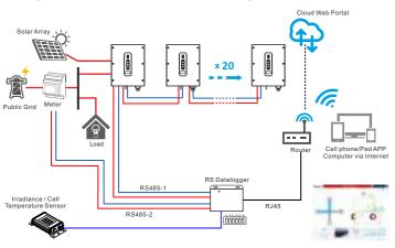
If needed, the energy meter can be installed on the load side, as an alternative to the grid side. In this case, the RS Datalogger must be configured as "Meter on load".
